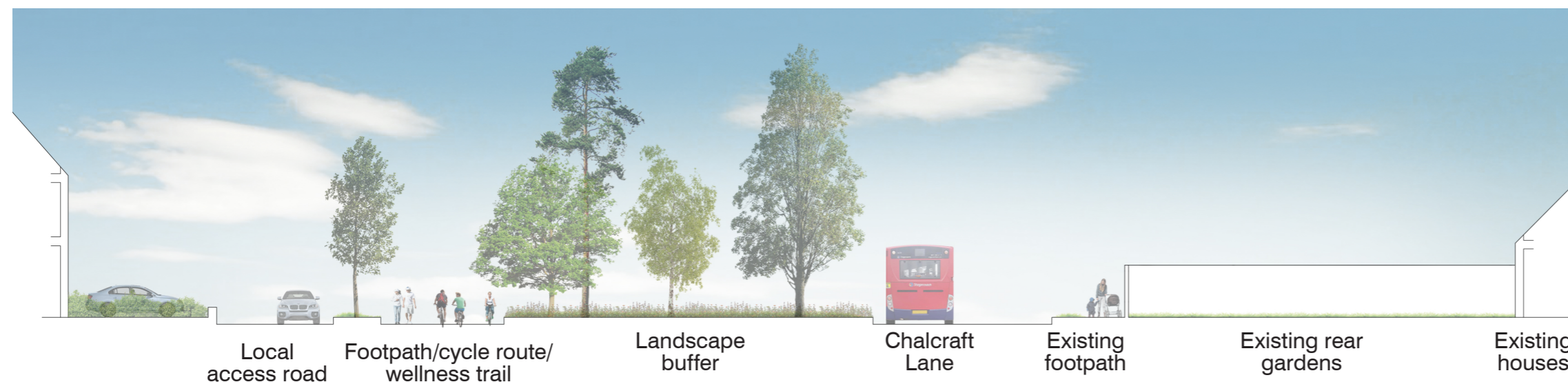
Indicative Cross Section 3 - residential to existing residential across Chalcraft Lane, showing tertiary local access road, shared footway/cycle paths, trees/landscape buffer, Chalcraft Lane and existing back gardens
